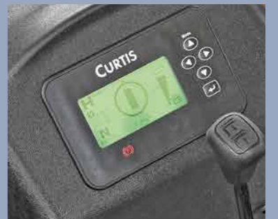
Instrument can display the steering angle and direction Synchronously
