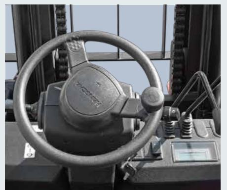
The design of steering wheel of small diameter and electro-hydraulic reversing as well as the car-type double-handle combination switch will greatly improve the driving comfort.
