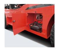
Battery compartment is easy to open for easy maintenance.
