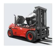
Thanks to the unique design, cab can be tilt without any tools, major service items can be reached easily by tilting the cabin, maximized access is possible.
